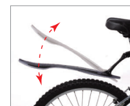
Mudguard Angle Adjustable
